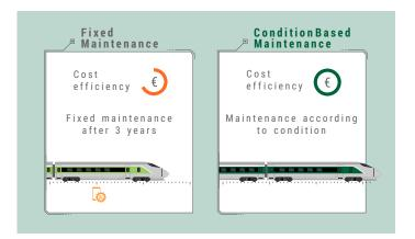
Since 01/03/2022 our vacuum toilet systems can be optionally equipped or upgraded with a function to visualize the need for a service. This option is available as "CBM – Condition Based Maintenance".
